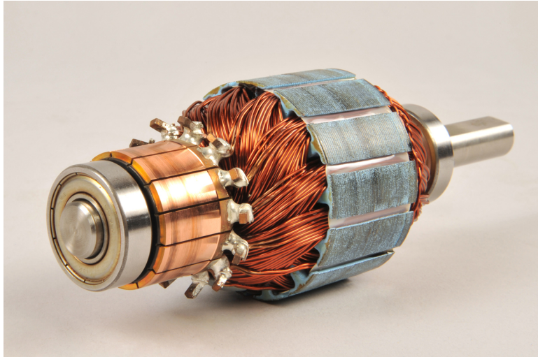
Figure 22. In real dc machines, the armature (rotor) is made up of several wire loops and the commutator has several segments.
